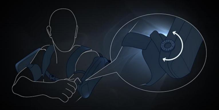
The assistance level can be **easily set by the worker** to quickly adapt to the ongoing activity with no need to remove the device.
